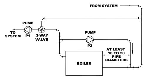
Figure 1 By-Pass Piping Using Three-Way Valve – Single Boiler
